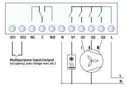
2-pipe ON/OFF 3-wire valve (220VAC); 1-3 speeds fan;
