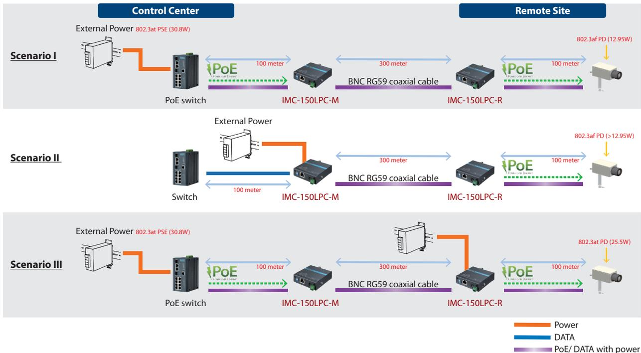
Note1: Advantech uses RG59 coaxial cables of Belden's 551945 010100, with the DCR conductor resistance value of 15 Ohm/1000ft to conduct tests. The transmitted output power and distance depends on resistance value of coaxial cables installed at field sites.
