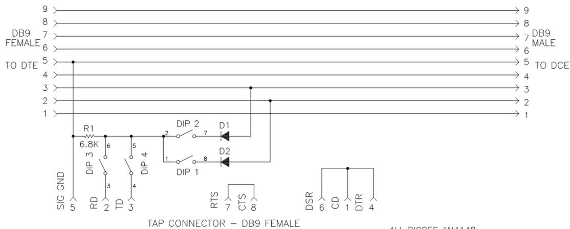
REV1-ADDED R1 FOR HIGHER BAUDRATE SUPPORT (UP TO 115.2K) NEWER PC HAD PROBLEM PULLING LINE DOWN OR TO -10V
