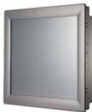
Changing to a solid-state HMI panel removes all of those components *and their associated wiring* and the failure points from each of the terminations of those wires. All that's left is the VFD, the contactors and the HMI panel. Operator panel construction and installation time was reduced as much as 90 percent in cases where the panel controls were complex.
